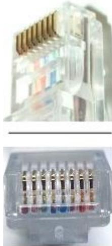
7. Place the wired plug into the crimping tool. Give the handle a firm squeeze. You should hear a ratcheting noise as you continue. Once you have completed the crimp, the handle will reset to the open position. To ensure all pins are set, some prefer to double-crimp by repeating this step.
