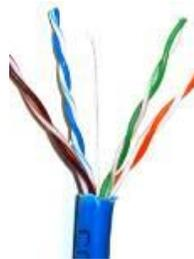
2. Inspect the newly revealed wires for any cuts or scrapes that expose the copper wire inside. If you have breached the protective sheath of any wire, you will need to cut the entire segment of wires off and start over at step one. Exposed copper wire will lead to cross-talk, poor performance or no connectivity at all. It is important that the jacket for all network cables remains intact.
