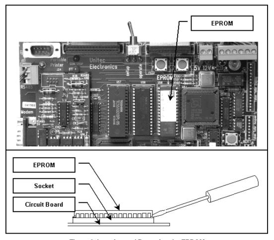
Figure 3. Locating and Removing the EPROM
