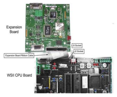
Figure 2. Expansion and CPU Board Layout
