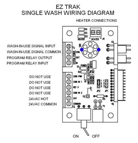
Figure 6. Interface Board Connections
